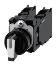
Selector switch, illuminable, 22 mm, round, plastic, white, selector switch, short, 3 switch positions I-O-II, latching, 10:30h/12h/13:30h, with holder, 2 x 1 NO+1 NC, spring-type terminal, with laser labeling, upper case and lower case, always upper case at beginning of line
