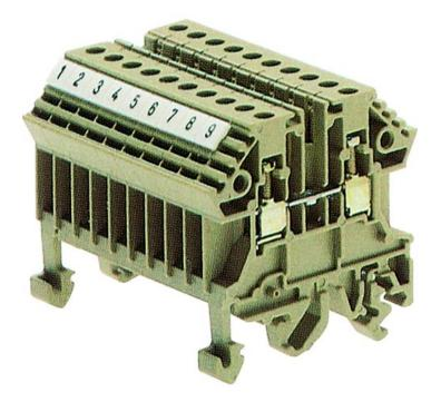
Feed-through terminal/block variant, Screw connection, Mounting type:Mounting rail TS 35/7.5 and TS 32, Rated cross-section: 2.5 mm<sup>2</sup>, Colour: Beige
