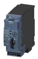
SIRIUS Compact load feeder DOL starter for IO-Link 690 V 24 V DC 8...32 A IP20 Connection main circuit: plug-in, without terminals Connection control circuit: Spring-type terminal
