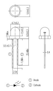
Note: Tolerances unless dimensions ±0.25mm
