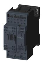
power contactor, AC-3 25 A, 11 kW / 400 V 1 NO + 1 NC, 230 V AC, 50 / 60 Hz, 3-pole, Size S0, Spring-type terminal
