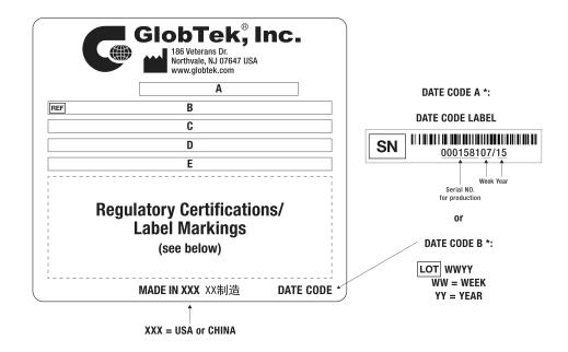
A=ICT / ITE / Medical Power Supply B=P/N: (料号) WR95D1110CCPIMFR6B C=Model (型号) GTM86101-1009-W2U D=Input (输入)100-240V~, 50-60Hz, 0.3A E=Output (输出)9.0 V === 1.11 A, 10.00W
