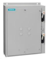
Duplex starter w/o alternator, Size 1, Three phase full voltage, Solid-state overload relay, OLR amp range 0.75-3.4A, 24VAC 50-60Hz coil, Combination type, Two 3A circuit breakers, Enc NEMA type 4 painted steel, Water/dust tight for outdoors
