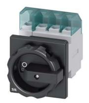
SENTRON, Switch disconnector 3LD, main switch, 4-pole, lu: 32 A, Operating power / at AC-23 A at 400 V: 11.5 kW, front-mounted, rotary operating mechanism, black, central mounting 22.5 mm of the handle
