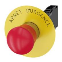
EMERGENCY STOP mushroom pushbutton, 22 mm, round, metal, shiny, red, 40 mm, positive latching, acc. to EN ISO 13850, rotate-to-unlatch, with yellow backing plate, inscription: Arrêt d'urgence, with holder, 1 NO+1 NC, screw terminal, Z=20-unit packaging
