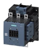
power contactor, AC-3 115 A, 55 kW / 400 V AC (50-60 Hz) / DC operation 110-127 V AC/DC auxiliary contacts 2 NO + 2 NC 3-pole, frame size S6 busbar connections drive: conventional spring-loaded terminal
