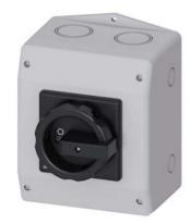
SENTRON, Switch disconnector 3LD, main switch, 6-pole, lu: 32 A, Operating power / at AC-23 A at 400 V: 11.5 kW, molded-plastic encapsulation for metric screw connection, 1 NC, 1 NO, rotary operating mechanism, black
