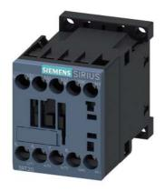
power contactor, AC-3 9 A, 4 kW / 400 V 1 NC, 24 V DC, 0.7-1.25\*US with integrated suppressor diode 3-pole, size S00, screw terminal suitable for PLC outputs not expandable with auxiliary switch
