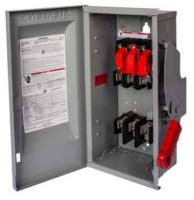
Siemens Low Voltage Circuit Protection Heavy Duty Safety Switches. Type: ENCLOSED, SAFETY SWITCH Std: UL V. Rating: 600V A. Rating: 100A No. Of Poles: 3P F. Rating: 60Hz Action: SINGLE THROW Material: 304SS Enclosure: TYPE 12. 2-3 point mounting holes. Insulation: YES O. Cycles: 10000 O. Temperature: (-20F-120F) AMBIENT TEMPERATURE Environmental Conditions: INDUSTRIAL
