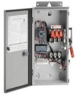
Slim Line Pump Control Panel NEMA size 1 Three phase full voltage Solidstate overload relay OLR amp range 5.5-22A 220/230V 50/60Hz Coil 30A fusible disconnect 30A/250V fuse clip 1NC / 1NO auxiliary contacts HOA Sel. Sw. <(>&<)> Start/Stop 3-point power terminal block 3-point control terminal block 3-point ground lug Enclosure NEMA type 3/3R Weather proof outdoor use
