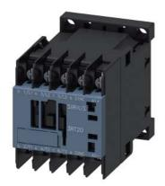
Power contactor, AC-3 7 A, 3 kW / 400 V 1 NC, 24 V DC 3-pole, Size S00 ring cable lug connection
