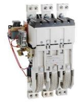
Mechanically held lighting contactor, Contactor amp rating 400A, 0 N.C. / 3 N.O. poles, 220VAC 50HZ/240VAC 60HZ coil, Non-combination type, Enclosure NEMA type (open), No enclosure
