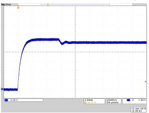
Zero to 10 A power ON curve using pin 8 to control the output.
