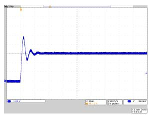
Zero to 3 A power ON curve using pin 8 to control the output.
