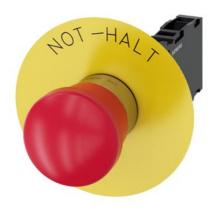
EMERGENCY STOP mushroom-type actuator, 22 mm, round, metal, shiny, red, 40 mm, positive latching, according to EN ISO 13850, pull-to-unlatch mechanism, with yellow backing plate, inscription: NOT-HALT, with holder, 1 NO+1 NC, screw terminal, Z=20-unit packaging
