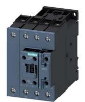
Contactor, 2NO + 2NC, AC-3, 22 kW, 110 V AC, 50 Hz, 4-pole, 2NO + 2NC, Size S2, Screw terminal 1 NO + 1 NC integrated
