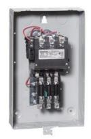
Non-reversing motor starter, Size 3 1/2, Three phase full voltage, Amb. compensate bimetal OLR, Contactor amp rating 115A, 110V 50Hz / 120V 60Hz coil, Non-combination type, Enclosure type 1, Indoor general purpose use
