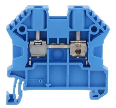
Feed-through terminal, Screw connection, Mounting type: Mounting rail TS 35/7.5, Rated cross-section: 4 mm<sup>2</sup>, Width: 6 mm, Colour: Blue
