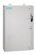
Non-reversing motor starter, Size 3, Three phase full voltage, Solid-state overload relay, OLR amp range 25-100A, 24VAC 50-60Hz coil, Combination type, 100A non-fusible disconnect, Encl NEMA type 4X 304 S-Steel, Water/dust tight noncorrosive, Extra-wide enclosure
