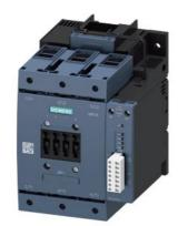
power contactor, AC-3 115 A, 55 kW / 400 V AC (50-60 Hz) / DC operation 200-277 V AC/DC auxiliary contacts 1 NO + 1 NC 3-pole, frame size S6 with box terminals drive: electronic with PLC / SIMOCODE - interface and remaining lifetime signal
