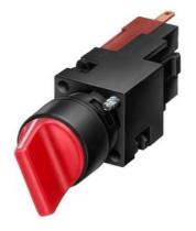
Selector switch, 16 mm, round, plastic, green, 3 switch positions I-O-II, latching, Actuating angle 2 x 62 degree, 1 NO, 1 NO
