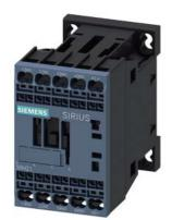
Contactor relay for railway 3 NO + 1 NC DC 72-125V, 0,7...1,25\*US, with integrated varistor Size S00, Spring-type terminal suitable for PLC outputs
