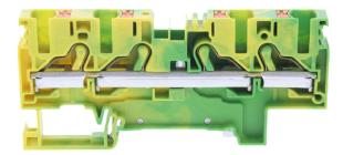
Protective earth terminal, Push-in connection, Mounting type: Mounting rail TS 35/7.5, Rated cross-section: 6 mm<sup>2</sup>, Width: 8.1 mm, Colour: Green-yellow
