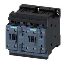
Reversing contactor assembly AC-3, 15 kW/400 V, 24 V DC 3-pole, Size S0 screw terminal electrical and mechanical Interlock 2 NO integrated
