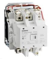
Mechanically held lighting contactor, Contactor amp rating 100A, 0 N.C. / 2 N.O. poles, 24VAC 60HZ coil, Non-combination type, Enclosure NEMA type (open), No enclosure
