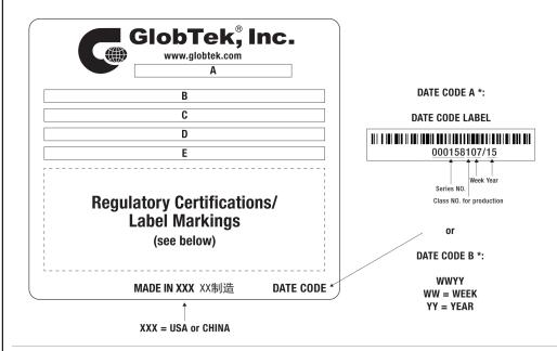
A=DC/DC Switching Power Supply B=P/N: (料号) DR6SM4800USBC-USBAPD C=Model (型号) GTD9X0240-24PD D=Input (输入)12-24 Vdc, 2.5 A
