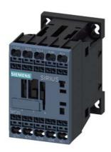
power contactor, AC-3 12 A, 5.5 kW / 400 V 1 NC, 125 V DC 0.7-1.25\*US with integrated suppressor diode 3-pole, size S00 spring-type terminal suitable for PLC outputs not expandable with auxiliary switch
