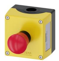
Enclosure for command devices, 22 mm, round, Enclosure material plastic, Enclosure top part yellow, 1 control point plastic, Control point in center, A=EMERGENCY STOP mushroom pushbutton red, 40 mm, rotate-tounlatch, 1 NC, 1NC, screw terminal, floor mounting, 1xM20 each on top and bottom
