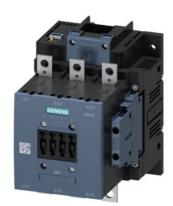
Traction contactor, AC-3 150 A, 75 kW / 400 V Coil 24 V DC x (0.7-1.25) PLC input 24-110 V DC Auxiliary contacts 2 NO + 2 NC 3-pole size S6 Busbar connections Coil connection: screw terminal
