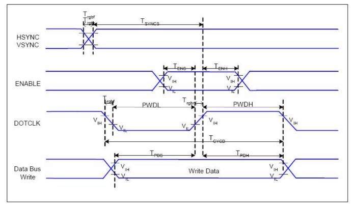
Figure 6.1: Parallel RGB Interface Timing Diagram
