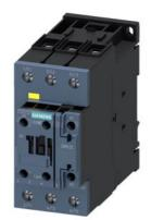
contactor, AC-3, 40 A/400 V/60  $^\circ C$  S2, 3-pole, 21-33 V AC/DC, F-PLC-IN, with varistor, 1 NC, screw terminal
