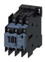
Traction contactor, AC-3 32 A, 15 kW / 400 V 1 NO + 1 NC with solid-state operating mechanism 24 V DC, 0.7-1.25\* Us with integrated varistor 3-pole, size S0 ring cable lug connection
