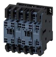
Reversing contactor assembly AC-3, 5.5 kW/400 V,AC230V,50/60Hz 3-pole, Size S0 Spring-type terminal electrical and mechanical interlock
