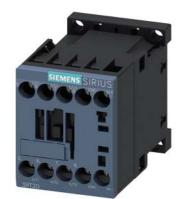
power contactor, AC-3 12 A, 5.5 kW / 400 V 1 NC, 230 V DC 3-pole, Size S00 screw terminal
