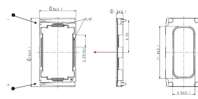
Note: Positive voltage on pin '+' moves membrane in direction of red arrow!
