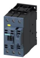
contactor, AC-3, 40 A/400 V/60  $^\circ C$  S2, 3-pole, 83-150 V AC/DC, F-PLC-IN, with varistor, 1 NC, spring-loaded terminal
