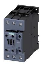
Contactor, 25 hp, 460 / 575 V 1 NO + 1 NC, 110 V AC, 50 Hz / 120 V, 60 Hz, 3-pole, Size S2, screw terminal NEMA size 2
