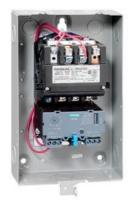
Non-reversing motor starter, Size 1 3/4, Three phase full voltage, Solid-state overload relay, OLR amp range 10-40A, 24VAC 50-60Hz coil, Non-combination type, Enclosure type 1, Indoor general purpose use, Standard width enclosure
