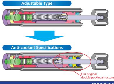
In a normal absorber, adhering liquid is pushed inside with each stroke. This can block the accumulator and the flow of oil, ultimately preventing the rod from inserting or causing other trouble.
