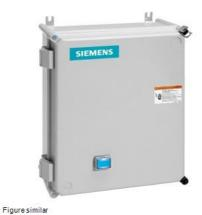
Non-reversing motor starter, Size 2 1/2, Three phase full voltage, Amb. compensate bimetal OLR, Contactor amp rating 60A, 24VAC 50-60Hz coil, Non-combination type, Enclosure type 4X fiberglass, Water/dust tight noncorrosive
