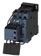
Capacitor contactor, AC-6b 25 kVAr, / 400 V 1 NO + 2 NC, 50-60 Hz AC 95-130 V DC 3-pole, Size S0 screw terminal
