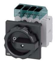
Load disconnector 3LD3, lu 63 A Main switch 3-pole + N Rated operating capacity at AC-23 A at 400V 22.0 kW Front plate mounting Basic switch with Central hole mounting 22.5mm Toggle drive black 66x66 mm with auxiliary switch 1OE + 1S
