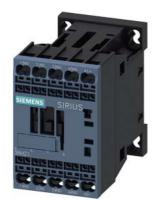
Coupling contactor relay, 3 NO + 1 NC, 24 V DC, 0.7 ... 1.25\* US, Size S00, Spring-type terminal suitable for PLC outputs
