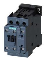
power contactor, AC-3 12 A, 5.5 kW / 400 V 1 NO + 1 NC, 24 V DC with plugged-in diode combination, 3-pole Size S0, screw terminal
