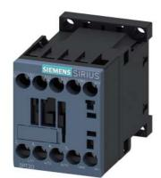
power contactor, AC-3 7 A, 3 kW / 400 V 1 NO, 24 V DC 0.7-1.25\* US, with diode integrated, 3-pole, suitable for PLC outputs not expandable with auxiliary switch
