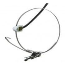
Temperature probe with Pt1000 sensor. Surface probe for tubing and flat surface, range from -30 to +130°C, 5 meters cable, IP65. Without connector.
