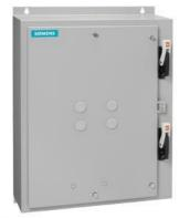
Duplex starter w/o alternator Size 0 Three phase full voltage Solid-state overload relay OLR amp range 0.25-1A 208VAC 60Hz Coil Combination type Two 30A disconnect switches Enclosure NEMA type 1 Indoor general purpose use
